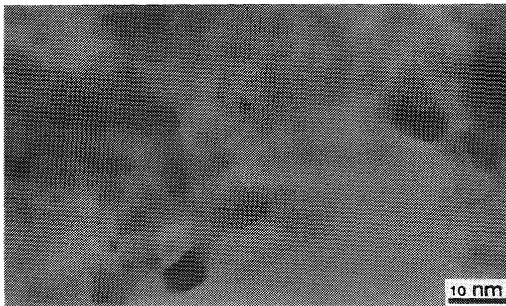
FIG. 7. TEM micrograph of 3.0 wt.% Pt-3.0 wt.% Re/ \gamma -Al 2 O 3 catalyst. The particle number density is higher than that in EUROPT-3 and EUROPT-4.
